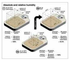
Here's where it gets interesting! Air at 70°F can hold twice as much moisture as air at 50°F. If we cool a sample of air at 70°F with 50% relative humidity to 50°F, the relative humidity rises to 100%. If the temperature falls to 49°F, we get condensation. And that can be a problem ...
