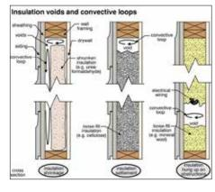
Loose-fill insulation that is blown or poured in can also settle, creating voids at tops of wall cavities, for example. Where insulation is poured or blown into wall cavities, voids may develop if the insulation gets hung up on obstructions partway down the cavity. Voids may also develop in insulations that shrink. Urea-formaldehyde foam insulation sometimes shrank dramatically after it was installed, reducing its R-value.
