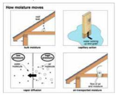
Bulk moisture is the most visible and significant source of water damage in houses. Air transported moisture is second. Vapor diffusion and capillary action are relatively minor issues. Let's look at air-transported moisture.
