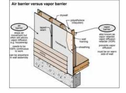
*As you can see, a vapor diffusion retarder has fewer* functions and is less critical than an air barrier. Let's look at air barriers first.
